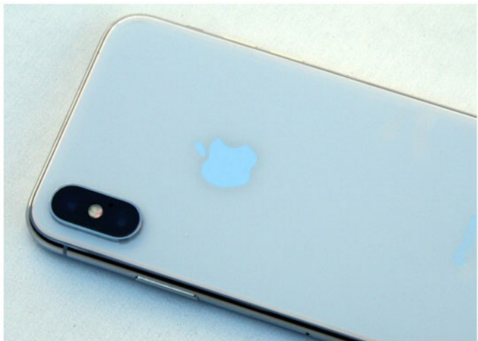
The back of the iPhone X uses glass to allow for wireless charging.
